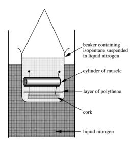
the specimen. One the specimen is frozen it is essential that it is handled only with cooled instruments. Gripping the specimen with forceps at room temperature will cause partial thawing which again induces artefact. For long term storage immersion in a Linde flask of liquid
