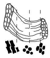
Elongated profiles are obtained in oblique sections. True transverse sections are required for accurate measurement of fibre diameter and comparison of fibre size.
